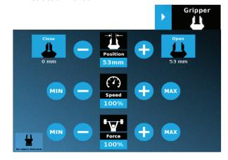
Depending on the PolyScope settings used, the Gripper position measurements can either display in metric or imperial units.
