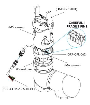
\*The dowel pin is meant to have a tight fit on the robot side and a slip fit on the effector side of the assembly.
