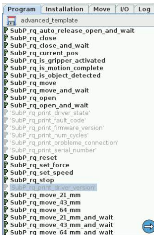
Fig. 4-21: Older program's subprograms to suppress or rename to use with URcaps package.
